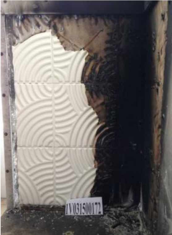
Fig4. Long wing (left) after SBI test
