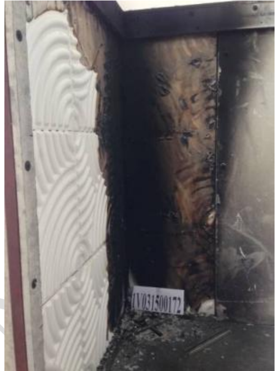
Fig5. Short wing (right) after SBI test
