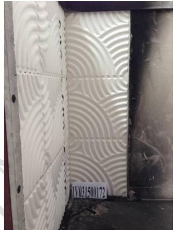
Fig3. Short wing (right) before SBI test
